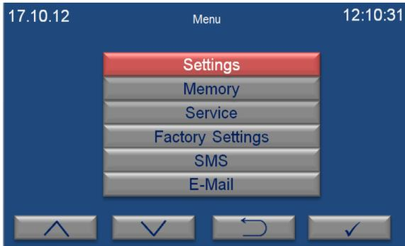
Main menu page appears when the password is approved by pushing enter key (F4). Submenu can be selected by using the value increase and decrease keys. The selected menu becomes red and enter key (F4) is pushed to enter this menu.
