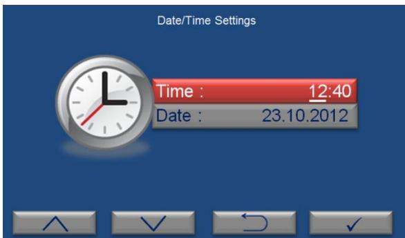
“Date/Time Settings” submenu is selected on the settings page by the value increase (F1) and decrease (F2) keys. The page shown on the left appears when enter key (F4) is pushed. Time is shown in the format of “hour:minute” and the cursor is on hour part when “Date/Time Settings” page comes to the screen. Hour is adjusted by pushing the value increase (F1) and decrease (F2) keys. In order to continue to adjust, push enter key (F4).
